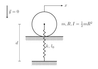
Analysis of the scheme allows to claim its number of degrees of freedom which is 1
